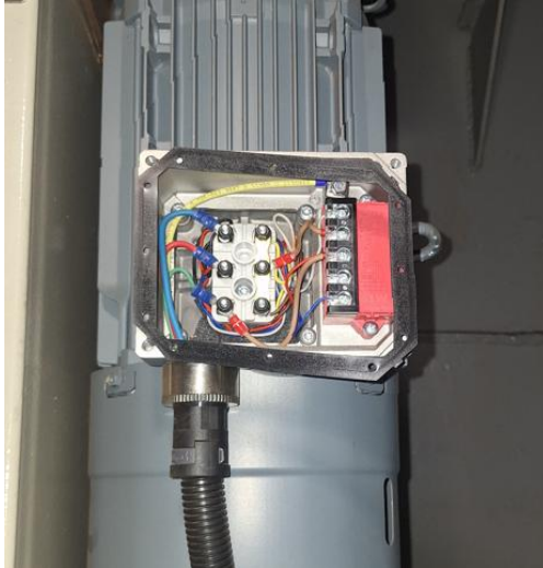
Motor setup according to voltage input
