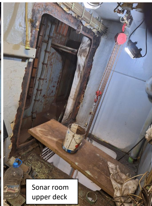
Works done on sonar room to install the hull unit (upper deck)
